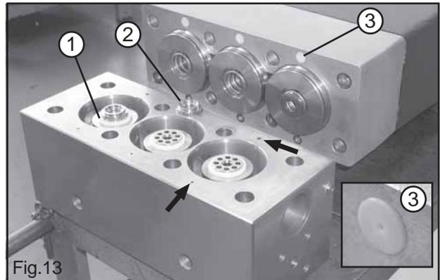
When removing the head from the pump pay attention to the valve seats (1, Fig.13) and the suction valve disks (2 Fig.13) which may fall off the head.
