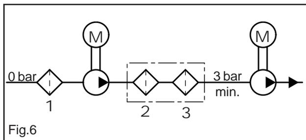
The filters should be installed as close as possible to the pump, allow easy inspection and have the following specifications:
