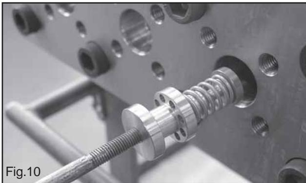
Once removed, take out the delivery valve guide with the spring and valve disk. An M10 threaded bolt to be used as a simple extractor would help the operation (see Fig.10).
