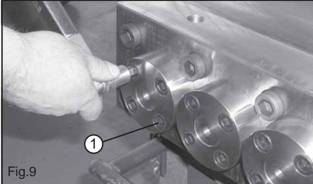
In order to have access to the delivery valves loose the 12 valve cover screws (1, Fig.9) and remove the valve covers.
