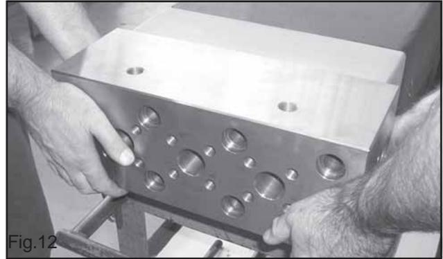
Remove the pump head (Fig.12).
