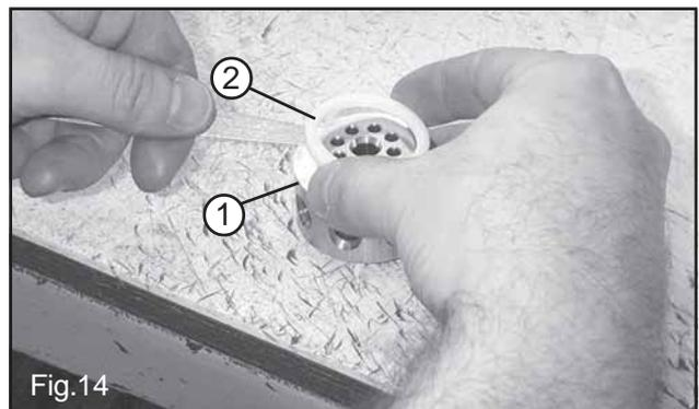
Remove the valve seats (1, Fig.14) from the head, check them for wear and replace if necessary.
