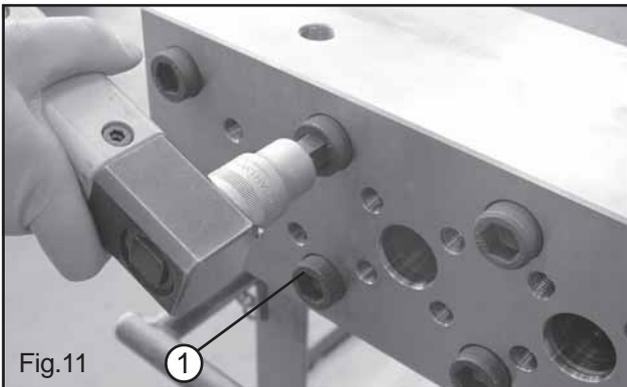
Loose and remove the 8 head screws (1 Fig.11).
