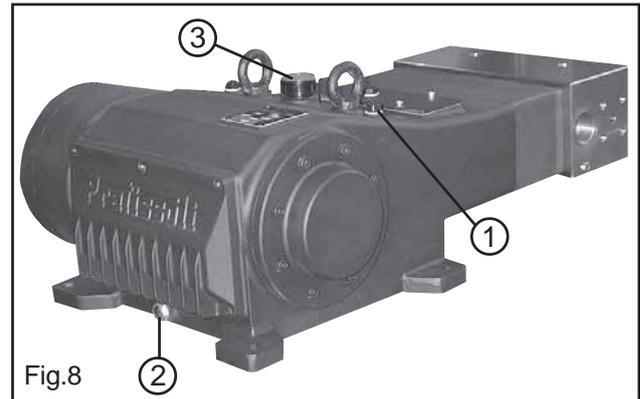
If necessary, top up from the oil plug 3, Fig.8. Check the oil when cold and change the oil when still hot (pump still at working temperature). In order to drain the oil from the pump remove the magnetic plug 2, Fig.8. At every oil change clean the magnetic plug 2 Fig.8 and check the lower cover of Fig.7 for sediments or deposits.
